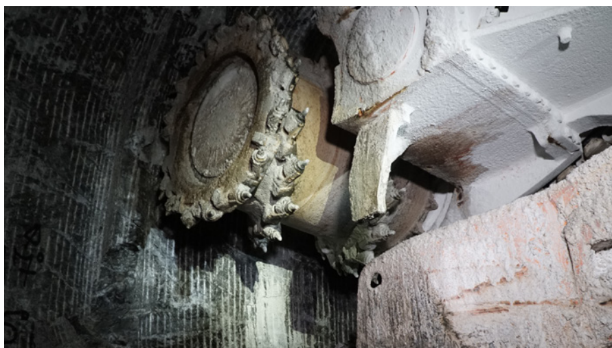
Photo 9. Continuous mining machine used to extract the polyhalite mineral from 1,200 m below ground in the polyhalite mine at Boulby, Yorkshire, UK. Photo: ICL, UK.
