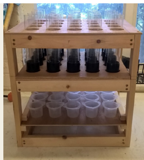
Photo 5. Leach columns used in experiment at University of Nottingham.
