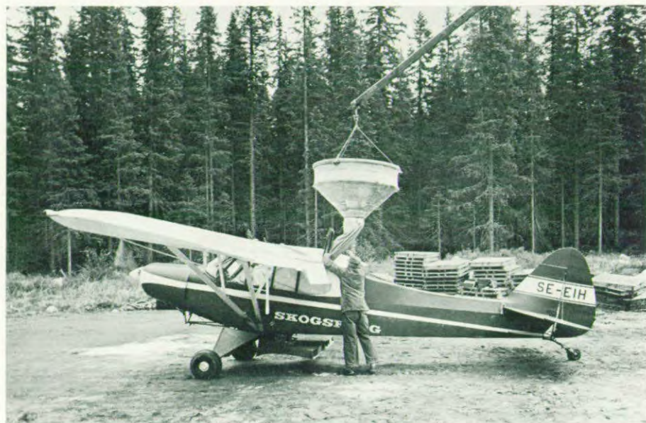
Fig. 2: Previously Piper Cub aircrafts were used, carrying 250 kg of fertilizer.
