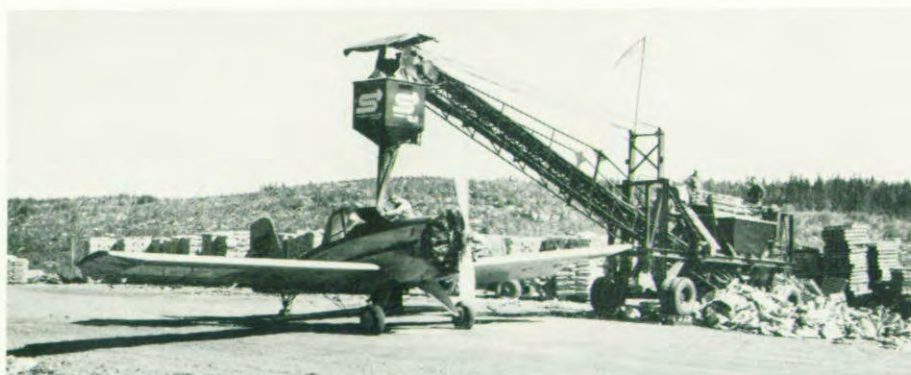
Fig.6: Loading 800 kg of Urea in Aero Commander Snow aircraft on SCA airstrip.
