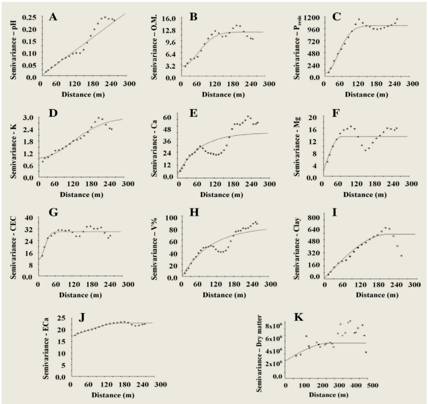
**Fig. 2.** Semi-variograms of pH (A); organic matter (B); available P (C); exchangeable K (D); Ca (E); Mg (F); cation exchange capacity (CEC) (G); base saturation-V% (H); clay (I); soil apparent electrical conductivity (ECa) (J); and dry matter yield (K) of a grazed alfalfa pasture in Brazil.
