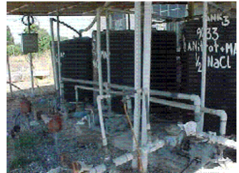
Fertigation system used in the mandarin experiment. The fertilizer (fertigation) tank also contains the salinization agent (NaCl). Photo by C. Kilic.
