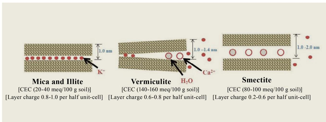
Fig. 1. Properties of four types of clay minerals often present in agricultural soils. Adapted from Wakeel *et al.*, 2013.
