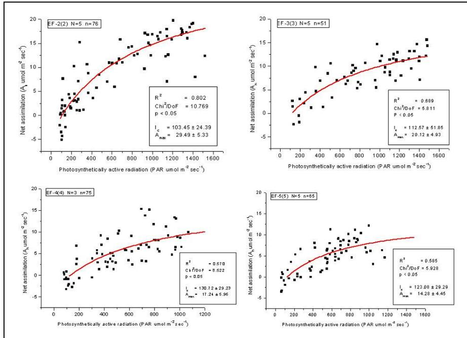
Figure 2 – Light-photosynthesis curves ( $A_n$ -PAR) in the experimental field (EF). Phenophase and leaf position e.g. EF 2(2), number of replicates (N), number of measuring points (n), coefficient of determination ( $R^2$ ), reduced chi-square value of fit, probability (p) and remarkable points of assimilation ( $I_c$ ,  $A_{max}$ ) are displayed.
