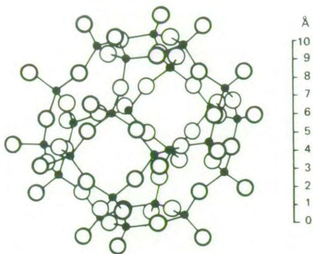
Fig. 3. Simplified tetrahedral arrangement in the framework structure of quartz (Mackenzie [1975]).
