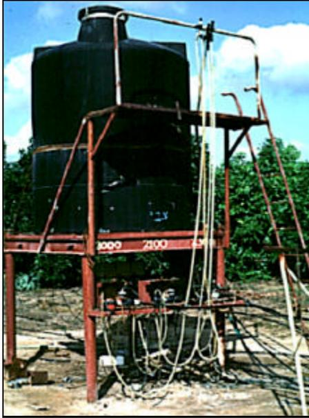
Fertigation: 5000 L stock solution tank with 3 parallel displacement pumps (Avocado plantation, Kibutz Givat Brenner, Israel).
